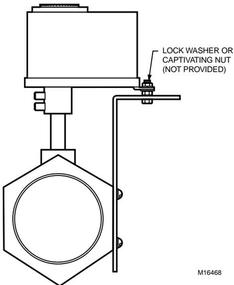
Fig. 4. Mounting ML7999 with mounting bracket accessory.
