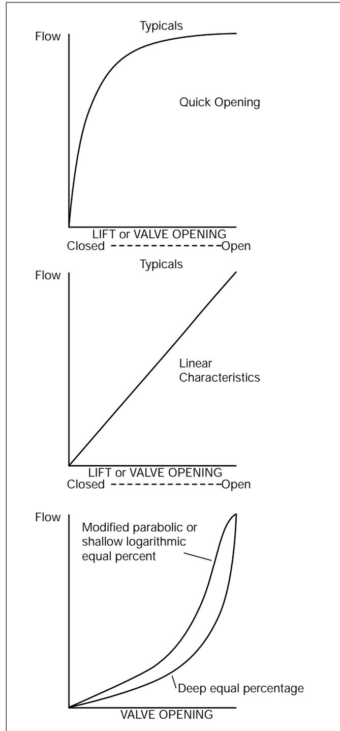
Figure 11 - Response curve of various valves
