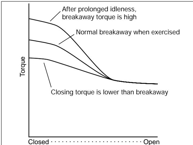
**Figure 36 - Torque requirements for ball and butterfly valves**
