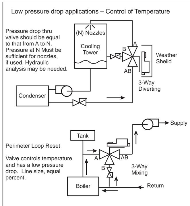
Figure 31 - Three-way valve applications controlling temperature
