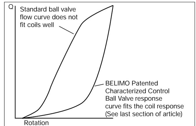
**Figure 5b - Belimo characterized control ball flow characteristic**
