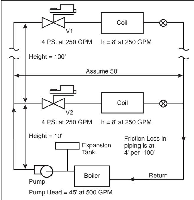
**Figure 32 - Boiler, pump and piping system**
