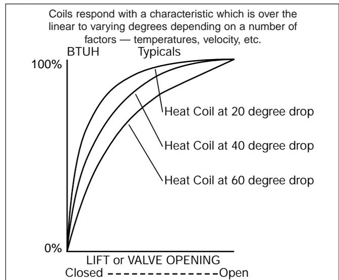
Figure 8 - Heat output of coil with varying temperatures
