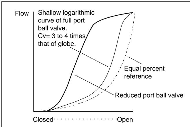
**Figure 4b - Full port ball valve flow characteristic**
