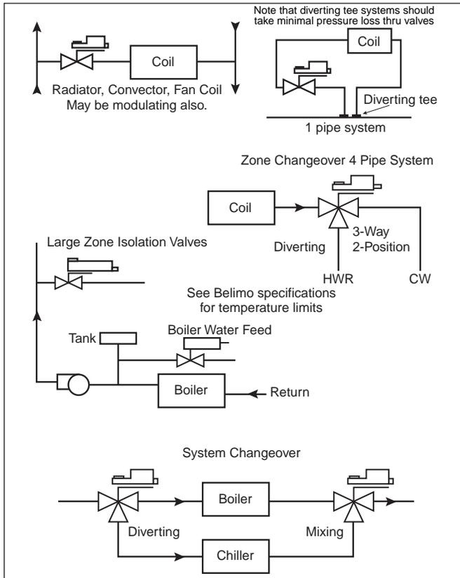
**Figure 26 - Two and three-way valves in 2-position application**
