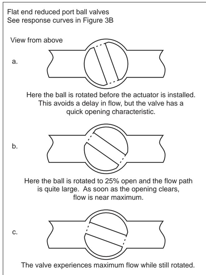
**Figure 3a - Flat end reduced port ball valve**
