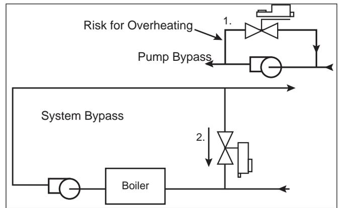
**Figure 30a - Bypass applications**
