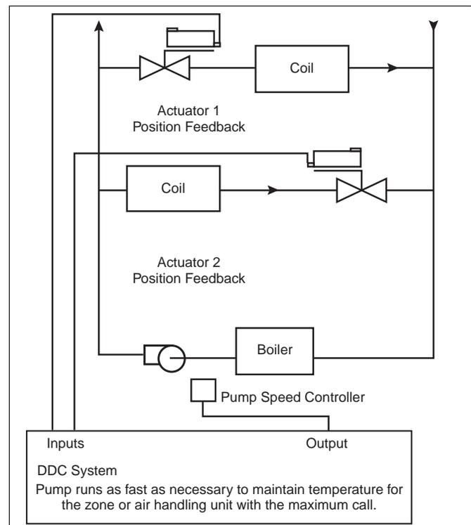
**Figure 29 - Variable flow high performance system**
