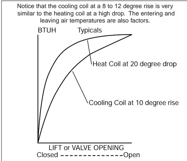
**Figure 9 - Response curve of cooling coil**
