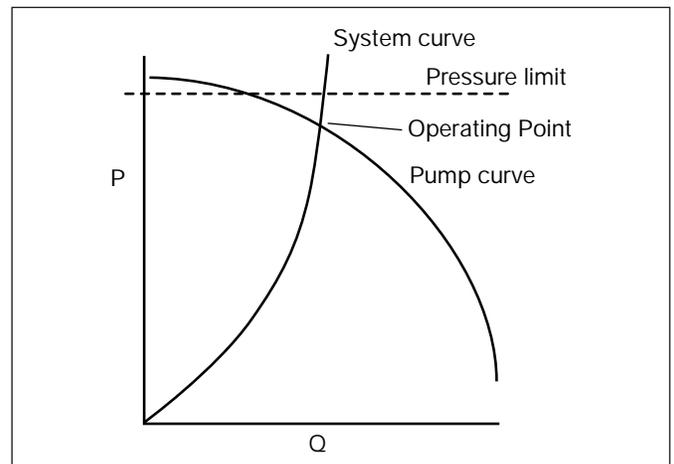
**Figure 30b - Pressure limit and operating point**
