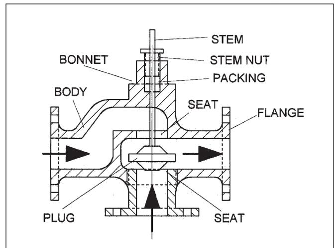
**Figure 2 - Three-way globe valve**
