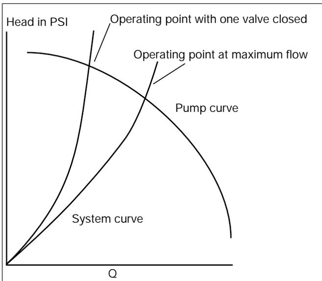
**Figure 28b - Variable flow systems pump curve**
