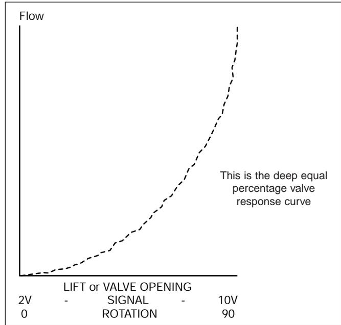
Figure 20 - Deep equal percentage valve response curve
