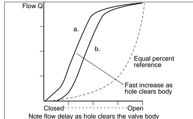
**Figure 3b - Reduced port ball valve flow characteristic**
