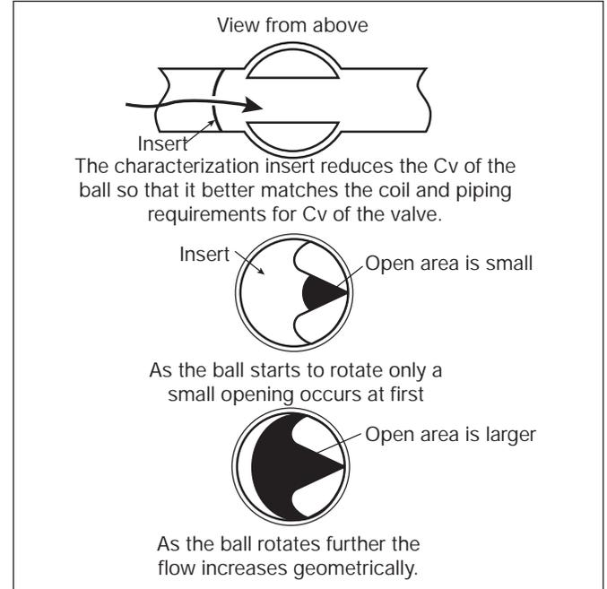
**Figure 5a - Belimo Characterized Control Ball Valve**
